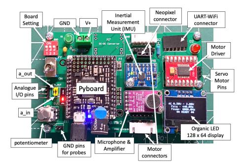
Unlike Electronics 1, you are **not** required to build electronics circuits on breadboard this year. Instead, you will be using a bespoke board (PCB) that I designed specifically for this module This unit is known as **PyBench Board** – it is my version of an electronic workbench which is programmed using MicroPython (uPy), and controlled via the USB serial port.
